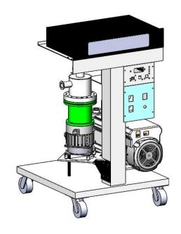
leakage or the probe failing to touch the electrode. At the same time, it can also provide effective refrigeration due to the vacuum insulation effect. In a high temperature test, it prevents the oxygen in the air from oxidizing the sample, thereby avoiding the electrical error of the sample as well as physical and mechanical deformation.
